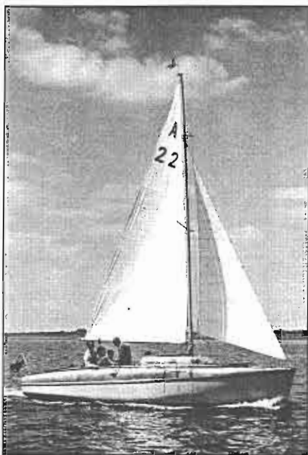
Above: An early example with varnished coachroof and decks. Note afterdeck for stowage of tender and, right, twin swing-keels which wind up flush with the bottom. Price Guide: £3,500-£5,500.
